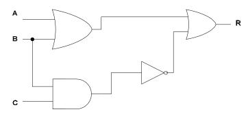
Looking at the circuit diagram from left to right and top to bottom, we see the following: the input to the final gate is (A+B) along with the result of  $\sim(BC)$
