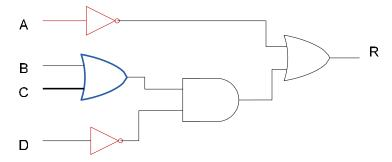
The topmost NOT gate takes A as input. Its out put is ~A. Below that is an OR gate which takes both B and C as input. Its output is contained in the expression (B+C). At the bottom in another NOT gate which can be represented at ~D.
